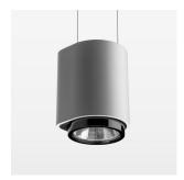
Suspended luminaire with LED, rated life of the LED L80/B10 50000 h (tambient 25°C), colour rendering index CRI > 82, chromaticity tolerance 2 SDCM (initial), reflector with oval light distribution pattern, 3D silicone lens to reduce the proportion of scattered light, reflector pure aluminium 99,99% in MIRO-Silver®, segmented, exchangeable reflector unit in high-sheen black plastic, with glass cover, luminaire housing die-cast aluminium, powdercoated, silver
