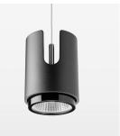
Suspended luminaire with LED, rated life of the LED L80/B10 50000 h (tambient 25°C), colour rendering index CRI > 90, chromaticity tolerance 2 SDCM (initial), reflector with oval light distribution pattern, 3D silicone lens to reduce the proportion of scattered light, reflector pure aluminium 99,99% in MIRO-Silver®, segmented, exchangeable reflector unit in high-sheen black plastic, with glass cover, luminaire housing die-cast aluminium, powder-coated, black
