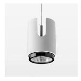
Suspended luminaire with LED, rated life of the LED L80/B10 50000 h (tambient 25°C), colour rendering index CRI > 80, chromaticity tolerance 2 SDCM (initial), reflector with oval light distribution pattern, 3D silicone lens to reduce the proportion of scattered light, reflector pure aluminium 99,99% in MIRO-Silver®, segmented, exchangeable reflector unit in high-sheen black plastic, with glass cover, luminaire housing die-cast aluminium, powdercoated, white
