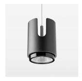
Suspended luminaire with LED, rated life of the LED L80/B10 50000 h (tambient 25°C), colour rendering index CRI > 96, chromaticity tolerance 2 SDCM (initial), reflector with oval light distribution pattern, 3D silicone lens to reduce the proportion of scattered light, reflector pure aluminium 99,99% in MIRO-Silver®, segmented, exchangeable reflector unit in high-sheen black plastic, with glass cover, luminaire housing die-cast aluminium, powdercoated, black
