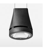
Suspended luminaire with LED, rated life of the LED L80/B10 > 50000 h, colour rendering index CRI > 80, chromaticity tolerance 2 SDCM (initial), reflector with circular light distribution pattern, reflector pure aluminium 99,99% in MIRO-Silver®, luminaire head die-cast aluminium, powder-coated, black
