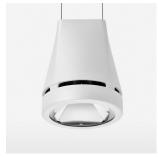
Suspended luminaire with LED, rated life of the LED L80/B10 > 50000 h, colour rendering index CRI > 80, chromaticity tolerance 2 SDCM (initial), reflector with circular light distribution pattern, reflector pure aluminium 99,99% in MIRO-Silver®, luminaire head die-cast aluminium, powder-coated, white
