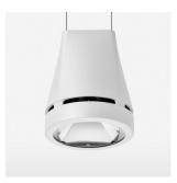
Suspended luminaire with LED, rated life of the LED L80/B10 > 50000 h, colour rendering index CRI > 82, chromaticity tolerance 2 SDCM (initial), reflector with circular light distribution pattern, reflector pure aluminium 99,99% in MIRO-Silver®, luminaire head die-cast aluminium, powder-coated, white
