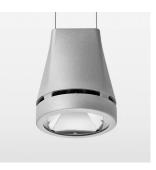
Suspended luminaire with LED, rated life of the LED L80/B10 > 50000 h, colour rendering index CRI > 80, chromaticity tolerance 2 SDCM (initial), reflector with circular light distribution pattern, reflector pure aluminium 99,99% in MIRO-Silver®, luminaire head die-cast aluminium, powder-coated, silver, separate driver unit
