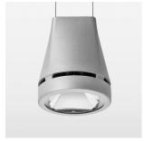
Suspended luminaire with LED, rated life of the LED L80/B10 > 50000 h, colour rendering index CRI > 90, chromaticity tolerance 2 SDCM (initial), reflector with circular light distribution pattern, reflector pure aluminium 99,99% in MIRO-Silver®, luminaire head die-cast aluminium, powder-coated, silver
