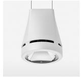
Suspended luminaire with LED, rated life of the LED L80/B10 > 50000 h, colour rendering index CRI > 70, chromaticity tolerance 2 SDCM (initial), reflector with circular light distribution pattern, reflector pure aluminium 99,99% in MIRO-Silver®, luminaire head die-cast aluminium, powder-coated, white
