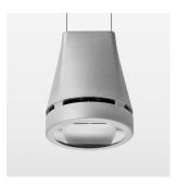
Suspended luminaire with LED, rated life of the LED L80/B10 > 50000 h, colour rendering index CRI > 70, chromaticity tolerance 2 SDCM (initial), reflector with oval light distribution pattern, reflector pure aluminium 99,99% in MIRO-Silver®, luminaire head die-cast aluminium, powder-coated, silver, separate driver unit
