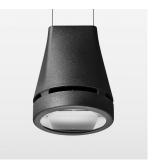
Suspended luminaire with LED, rated life of the LED L80/B10 > 50000 h, colour rendering index CRI > 80, chromaticity tolerance 2 SDCM (initial), reflector with oval light distribution pattern, reflector pure aluminium 99,99% in MIRO-Silver®, luminaire head die-cast aluminium, powder-coated, black
