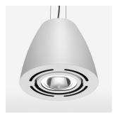
Suspended luminaire with LED, rated life of the LED L80/B10 > 50000 h, colour rendering index CRI > 82, chromaticity tolerance 2 SDCM (initial), reflector with circular light distribution pattern, reflector pure aluminium 99,99% in MIRO-Silver®, swivel angle +/-25°, luminaire housing sheet steel, powder-coated, white
