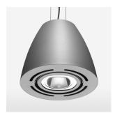
Suspended luminaire with LED, rated life of the LED L80/B10 > 50000 h, colour rendering index CRI > 82, chromaticity tolerance 2 SDCM (initial), reflector with circular light distribution pattern, reflector pure aluminium 99,99% in MIRO-Silver®, swivel angle +/-25°, luminaire housing sheet steel, powder-coated, silver
