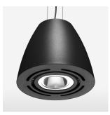
Suspended luminaire with LED, rated life of the LED L80/B10 > 50000 h, colour rendering index CRI > 82, chromaticity tolerance 2 SDCM (initial), reflector with oval light distribution pattern, reflector pure aluminium 99,99% in MIRO-Silver®, swivel angle +/-25°, luminaire housing sheet steel, powder-coated, black
