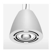
Suspended luminaire with LED, rated life of the LED L80/B10 > 50000 h, colour rendering index CRI > 80, chromaticity tolerance 3 SDCM (initial), reflector with circular light distribution pattern, reflector pure aluminium 99,99% in MIRO-Silver®, swivel angle +/-25°, luminaire housing sheet steel, powder-coated, white
