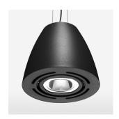
Suspended luminaire with LED, rated life of the LED L80/B10 > 50000 h, colour rendering index CRI > 90, chromaticity tolerance 2 SDCM (initial), reflector with oval light distribution pattern, reflector pure aluminium 99,99% in MIRO-Silver®, swivel angle +/-25°, luminaire housing sheet steel, powdercoated, black
