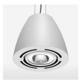
Suspended luminaire with LED, rated life of the LED L80/B10 > 50000 h, colour rendering index CRI > 90, chromaticity tolerance 2 SDCM (initial), reflector with circular light distribution pattern, reflector pure aluminium 99,99% in MIRO-Silver®, swivel angle +/-25°, luminaire housing sheet steel, powder-coated, white
