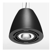
Suspended luminaire with LED, rated life of the LED L80/B10 > 50000 h, colour rendering index CRI > 80, chromaticity tolerance 2 SDCM (initial), reflector with circular light distribution pattern, reflector pure aluminium 99,99% in MIRO-Silver®, swivel angle +/-25°, luminaire housing sheet steel, powder-coated, black
