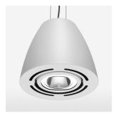
Suspended luminaire with LED, rated life of the LED L80/B10 > 50000 h, colour rendering index CRI > 90, chromaticity tolerance 2 SDCM (initial), reflector with circular light distribution pattern, reflector pure aluminium 99,99% in MIRO-Silver®, swivel angle +/-25°, luminaire housing sheet steel, powder-coated, white
