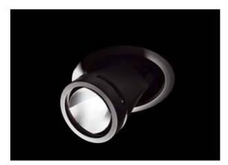
Semi-recessed luminaire with LED, chromaticity point tolerance 3 SDCM (initial), 2 SDCM for 927, 830, 835, 840, PearlWhite (initial), reflector 99.99% pure aluminium in MIRO-SILVER®, infinitely adjustable and pivotable luminaire head, built-in sheet steel housing, lightproof, die-cast aluminium luminaire head, powder coated, including glass cover, separate driver unit, luminaire colours black, silver, white, protection rating IP 20, protection class I, weight 2.0 kg
