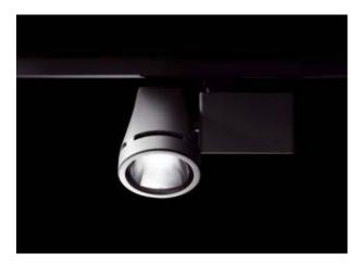
Surface-mounted spotlight with LED, passive cooling (up to 69 W), chromaticity point tolerance 3 SDCM (initial), 2SDCM for 927, 830, 835, 840, PearlWhite (initial), 99.99% pure aluminium reflector in MIRO-SILVER®, spotlight pivoted, adjustable luminaire head, die cast aluminium luminaire housing, powder-coated, including glass cover, multi-adapter, luminaire colours black, silver, white, protection rating IP 20, protection class I, weight 2.1 kg
