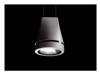
Suspended luminaire with LED, chromaticity point tolerance 3 SDCM (initial), 2 SDCM for 927, 830, 835, 840, PearlWhite (initial), 99.99% pure aluminium reflector in MIRO-SILVER®, die-cast aluminium luminaire head, powder coated, including glass cover, power supply via suspension cables, luminaire colours black, silver, white, protection rating IP 20, protection class I, weight 2.1 kg
