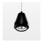
Suspended luminaire with LED, rated life of the LED L80/B10 > 50000 h, colour rendering index CRI > 90, chromaticity tolerance 2 SDCM (initial), reflector with circular light distribution pattern, reflector pure aluminium 99,99% in MIRO-Silver®, segmented and faceted, 3D lens silicon to reduce the proportion of scattered light, luminaire head die-cast aluminium, powdercoated, black, separate driver unit
