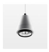
Suspended luminaire with LED, rated life of the LED L80/B10 > 50000 h, colour rendering index CRI > 80, chromaticity tolerance 2 SDCM (initial), reflector with circular light distribution pattern, reflector pure aluminium 99,99% in MIRO-Silver®, segmented and faceted, 3D lens silicon to reduce the proportion of scattered light, luminaire head die-cast aluminium, powder-coated, white
