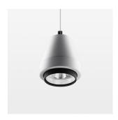
Suspended luminaire with LED, rated life of the LED L80/B10 > 50000 h, colour rendering index CRI > 96, chromaticity tolerance 2 SDCM (initial), reflector with circular light distribution pattern, reflector pure aluminium 99,99% in MIRO-Silver®, segmented and faceted, 3D lens silicon to reduce the proportion of scattered light, luminaire head die-cast aluminium, powder-coated, white
