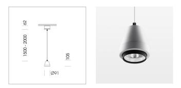
Suspended luminaire with LED, rated life of the LED L80/B10 > 50000 h, colour rendering index CRI > 90, chromaticity tolerance 2 SDCM (initial), reflector with circular light distribution pattern, reflector pure aluminium 99,99% in MIRO-Silver®,segmented and faceted, 3D lens silicon to reduce the proportion of scattered light, luminaire head die-cast aluminium, powder-coated, white
