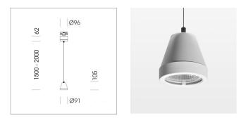
Suspended luminaire with LED, rated life of the LED L80/B10 > 50000 h, colour rendering index CRI > 90, chromaticity tolerance 2 SDCM (initial), reflector with circular light distribution pattern, reflector pure aluminium 99,99% in MIRO-Silver®,segmented and faceted, luminaire head die-cast aluminium, powder-coated, white
