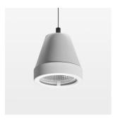
Suspended luminaire with LED, rated life of the LED L80/B10 > 50000 h, colour rendering index CRI > 80, chromaticity tolerance 2 SDCM (initial), reflector with circular light distribution pattern, reflector pure aluminium 99,99% in MIRO-Silver®, segmented and faceted, luminaire head die-cast aluminium, powder-coated, white
