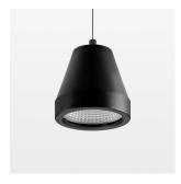
Suspended luminaire with LED, rated life of the LED L80/B10 > 50000 h, colour rendering index CRI > 96, chromaticity tolerance 2 SDCM (initial), reflector with circular light distribution pattern, reflector pure aluminium 99,99% in MIRO-Silver®, segmented and faceted, luminaire head die-cast aluminium, powder-coated, black
