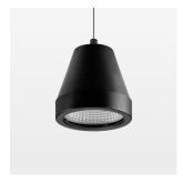
Suspended luminaire with LED, rated life of the LED L80/B10 > 50000 h, colour rendering index CRI > 80, chromaticity tolerance 2 SDCM (initial), reflector with circular light distribution pattern, reflector pure aluminium 99,99% in MIRO-Silver®, segmented and faceted, luminaire head die-cast aluminium, powder-coated, black
