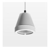
Suspended luminaire with LED, rated life of the LED L80/B10 > 50000 h, colour rendering index CRI > 80, chromaticity tolerance 2 SDCM (initial), reflector with circular light distribution pattern, reflector pure aluminium 99,99% in MIRO-Silver®, segmented and faceted, 3D lens silicon to reduce the proportion of scattered light, luminaire head die-cast aluminium, powder-coated, white
