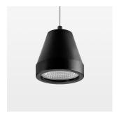
Suspended luminaire with LED, rated life of the LED L80/B10 > 50000 h, colour rendering index CRI > 90, chromaticity tolerance 2 SDCM (initial), reflector with circular light distribution pattern, reflector pure aluminium 99,99% in MIRO-Silver®, segmented and faceted, 3D lens silicon to reduce the proportion of scattered light, luminaire head die-cast aluminium, powder-coated, black
