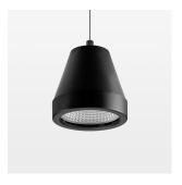
Suspended luminaire with LED, rated life of the LED L80/B10 > 50000 h, colour rendering index CRI > 80, chromaticity tolerance 2 SDCM (initial), reflector with circular light distribution pattern, reflector pure aluminium 99,99% in MIRO-Silver®, segmented and faceted, 3D lens silicon to reduce the proportion of scattered light, luminaire head die-cast aluminium, powder-coated, black
