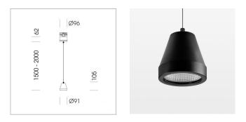
Suspended luminaire with LED, rated life of the LED L80/B10 > 50000 h, colour rendering index CRI > 96, chromaticity tolerance 2 SDCM (initial), reflector with circular light distribution pattern, reflector pure aluminium 99,99% in MIRO-Silver®,segmented and faceted, 3D lens silicon to reduce the proportion of scattered light, luminaire head die-cast aluminium, powder-coated, black
