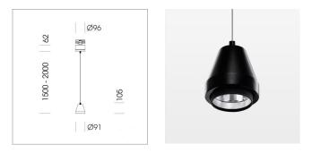
Suspended luminaire with LED, rated life of the LED L80/B10 > 50000 h, colour rendering index CRI > 80, chromaticity tolerance 2 SDCM (initial), reflector with circular light distribution pattern, reflector pure aluminium 99,99% in MIRO-Silver®,segmented and faceted, 3D lens silicon to reduce the proportion of scattered light, luminaire head die-cast aluminium, powder-coated, black
