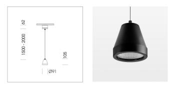
Suspended luminaire with LED, rated life of the LED L80/B10 > 50000 h, colour rendering index CRI > 96, chromaticity tolerance 2 SDCM (initial), reflector with circular light distribution pattern, reflector pure aluminium 99,99% in MIRO-Silver®,segmented and faceted, luminaire head die-cast aluminium, powder-coated, black
