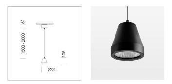
Suspended luminaire with LED, rated life of the LED L80/B10 > 50000 h, colour rendering index CRI > 90, chromaticity tolerance 2 SDCM (initial), reflector with circular light distribution pattern, reflector pure aluminium 99,99% in MIRO-Silver®,segmented and faceted, 3D lens silicon to reduce the proportion of scattered light, luminaire head die-cast aluminium, powdercoated, black
