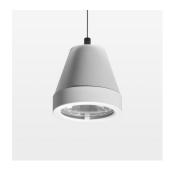
Suspended luminaire with LED, rated life of the LED L80/B10 > 50000 h, colour rendering index CRI > 96, chromaticity tolerance 2 SDCM (initial), rotation-symmetrical reflector with circular light distribution pattern, reflector pure aluminium 99,99% in MIRO-Silver®, segmented and faceted, 3D lens silicon to reduce the proportion of scattered light, luminaire head die-cast aluminium, powder-coated, white
