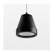
Suspended luminaire with LED, rated life of the LED L80/B10 > 50000 h, colour rendering index CRI > 90, chromaticity tolerance 2 SDCM (initial), reflector with circular light distribution pattern, reflector pure aluminium 99,99% in MIRO-Silver®, segmented and faceted, luminaire head die-cast aluminium, powder-coated, black
