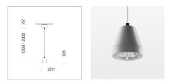
Suspended luminaire with LED, rated life of the LED L80/B10 > 50000 h, colour rendering index CRI > 80, chromaticity tolerance 3 SDCM (initial), rotation-symmetrical reflector with circular light distribution pattern, reflector pure aluminium 99,99% in MIRO-Silver®,segmented and faceted, 3D lens silicon to reduce the proportion of scattered light, luminaire head die-cast aluminium, powder-coated, silver
