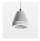
Suspended luminaire with LED, rated life of the LED L80/B10 > 50000 h, colour rendering index CRI > 90, chromaticity tolerance 2 SDCM (initial), reflector with circular light distribution pattern, reflector pure aluminium 99,99% in MIRO-Silver®, segmented and faceted, 3D lens silicon to reduce the proportion of scattered light, luminaire head die-cast aluminium, powdercoated, white
