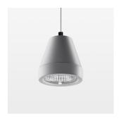
Suspended luminaire with LED, rated life of the LED L80/B10 > 50000 h, colour rendering index CRI > 80, chromaticity tolerance 3 SDCM (initial), rotation-symmetrical reflector with circular light distribution pattern, reflector pure aluminium 99,99% in MIRO-Silver®, segmented and faceted, 3D lens silicon to reduce the proportion of scattered light, luminaire head die-cast aluminium, powder-coated, silver
