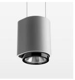
Suspended luminaire with LED, rated life of the LED L80/B10 50000 h (tambient 25°C), colour rendering index CRI > 70, chromaticity tolerance 2 SDCM (initial), reflector with oval light distribution pattern, 3D silicone lens to reduce the proportion of scattered light, reflector pure aluminium 99,99% in MIRO-Silver®, segmented, exchangeable reflector unit in high-sheen black plastic, with glass cover, luminaire housing die-cast aluminium, powder-coated, silver
