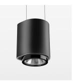
Suspended luminaire with LED, rated life of the LED L80/B10 50000 h (tambient 25°C), colour rendering index CRI > 90, chromaticity tolerance 2 SDCM (initial), reflector with oval light distribution pattern, 3D silicone lens to reduce the proportion of scattered light, reflector pure aluminium 99,99% in MIRO-Silver®, segmented, exchangeable reflector unit in high-sheen black plastic, with glass cover, luminaire housing die-cast aluminium, powder-coated, black
