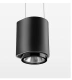
Suspended luminaire with LED, rated life of the LED L80/B10 50000 h (tambient 25°C), colour rendering index CRI > 80, chromaticity tolerance 2 SDCM (initial), reflector with oval light distribution pattern, 3D silicone lens to reduce the proportion of scattered light, reflector pure aluminium 99,99% in MIRO-Silver®, segmented, exchangeable reflector unit in high-sheen black plastic, with glass cover, luminaire housing die-cast aluminium, powder-coated, black
