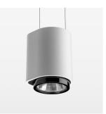
Suspended luminaire with LED, rated life of the LED L80/B10 50000 h (tambient 25°C), colour rendering index CRI > 80, chromaticity tolerance 2 SDCM (initial), reflector with circular light distribution pattern, reflector pure aluminium 99,99% in MIRO-Silver®, segmented and faceted, exchangeable reflector unit in high-sheen black plastic, with glass cover, luminaire housing die-cast aluminium, powder-coated, white Please order canopy and driver unit separatly
