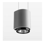
Suspended luminaire with LED, rated life of the LED L80/B10 50000 h (tambient 25°C), colour rendering index CRI > 80, chromaticity tolerance 2 SDCM (initial), reflector with circular light distribution pattern, reflector pure aluminium 99,99% in MIRO-Silver®, segmented and faceted, exchangeable reflector unit in high-sheen black plastic, with glass cover, luminaire housing die-cast aluminium, powder-coated, silver
