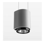
Suspended luminaire with LED, rated life of the LED L80/B10 50000 h (tambient 25°C), colour rendering index CRI > 80, chromaticity tolerance 2 SDCM (initial), reflector with oval light distribution pattern, 3D silicone lens to reduce the proportion of scattered light, reflector pure aluminium 99,99% in MIRO-Silver®, segmented, exchangeable reflector unit in high-sheen black plastic, with glass cover, luminaire housing die-cast aluminium, powdercoated, silver
