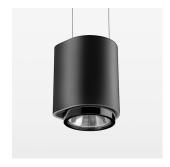
Suspended luminaire with LED, rated life of the LED L80/B10 50000 h (tambient 25°C), colour rendering index CRI > 95, chromaticity tolerance 2 SDCM (initial), reflector with oval light distribution pattern, 3D silicone lens to reduce the proportion of scattered light, reflector pure aluminium 99,99% in MIRO-Silver®, segmented, exchangeable reflector unit in high-sheen black plastic, with glass cover, luminaire housing die-cast aluminium, powdercoated, black
