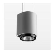
Suspended luminaire with LED, rated life of the LED L80/B10 50000 h (tambient 25°C), colour rendering index CRI > 95, chromaticity tolerance 2 SDCM (initial), reflector with circular light distribution pattern, 3D silicone lens to reduce the proportion of scattered light, reflector pure aluminium 99,99% in MIRO-Silver®, segmented and faceted, exchangeable reflector unit in high-sheen black plastic, with glass cover, luminaire housing die-cast aluminium, powder-coated, silver
