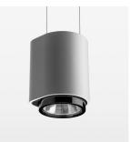
Suspended luminaire with LED, rated life of the LED L80/B10 50000 h (tambient 25°C), colour rendering index CRI > 95, chromaticity tolerance 2 SDCM (initial), reflector with oval light distribution pattern, 3D silicone lens to reduce the proportion of scattered light, reflector pure aluminium 99,99% in MIRO-Silver®, segmented, exchangeable reflector unit in high-sheen black plastic, with glass cover, luminaire housing die-cast aluminium, powder-coated, silver
